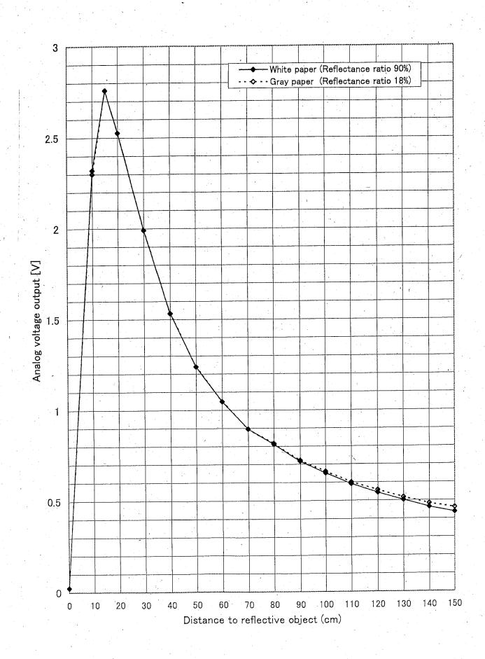
6-2 GP2Y0A02YK0F Example of output distance characteristics with the inverse of distance
