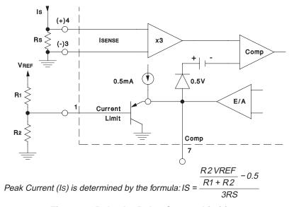
Figure 8. Pulse by Pulse Current Limiting
