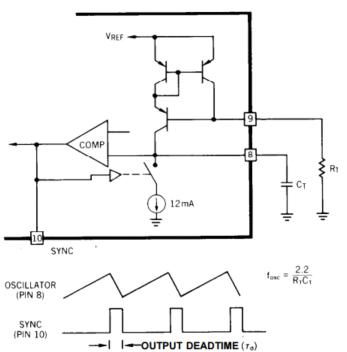
Figure 4. Oscillator Circuit
