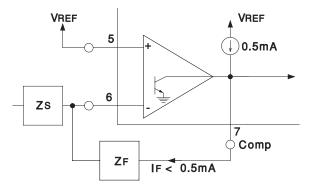
Error Amplifier can source up to 0.5mA.
