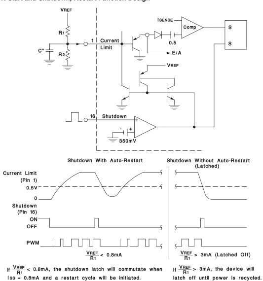
Figure 9. Soft-Start and Shutdown, Restart Functions
