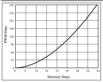
Figure 7 Gamma Correction (64 Steps)
