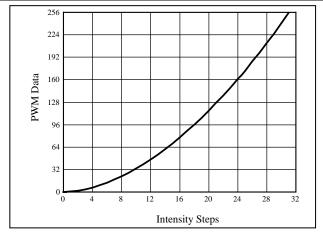
Figure 6 Gamma Correction (32 Steps)
