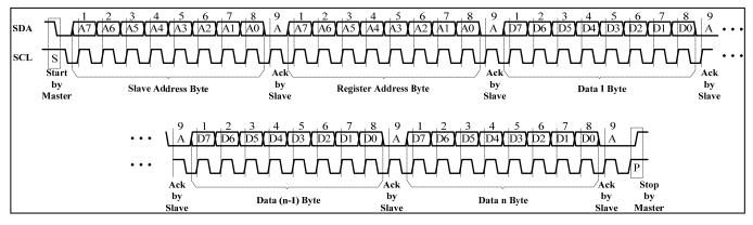
Figure 5 Writing to IS31FL3236A (Automatic Address Increment)
