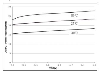
**Figure 8** V<sub>CC</sub> vs. Output PWM Frequency
