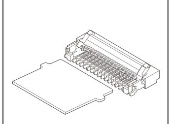
0.2mm pitch FVX connector for FPC has been developed for small portable equipment for which low profile and miniaturization are required. By using FPC with protrusions, the positioning accuracy of FPC is improved.
