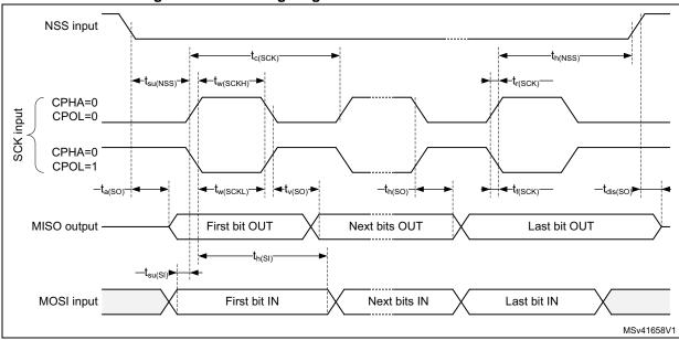
Figure 29. SPI timing diagram - slave mode and CPHA = 0
