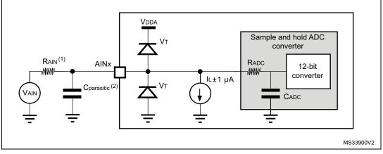
Refer to Table 52: ADC characteristics for the values of  $R_{AIN}$ ,  $R_{ADC}$  and  $C_{ADC}$ . 1.
