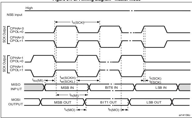
Figure 31. SPI timing diagram - master mode
