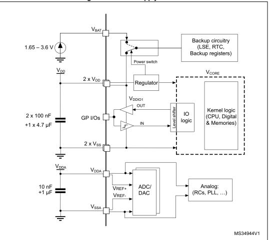
Figure 13. Power supply scheme
