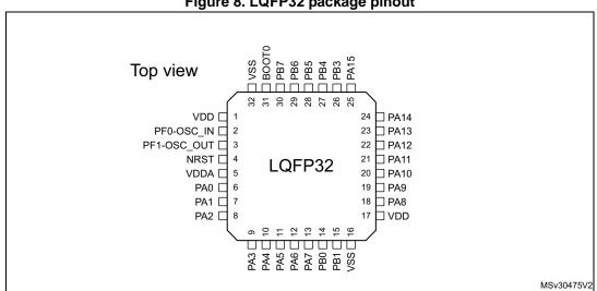
Figure 8. LQFP32 package pinout
