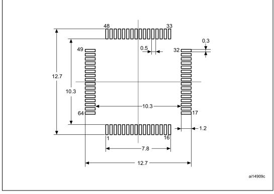
Figure 38. Recommended footprint for LQFP64 package
