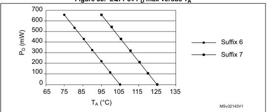
Figure 55. LQFP64 P<sub>D</sub> max versus T<sub>A</sub>
