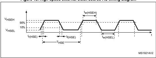
Figure 15. High-speed external clock source AC timing diagram
