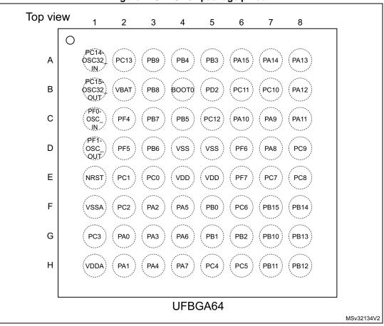
Figure 4. UFBGA64 package pinout
