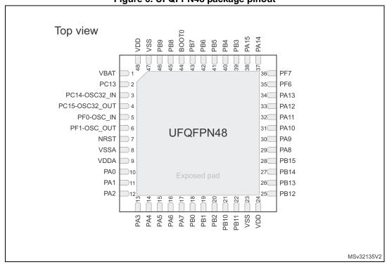
Figure 6. UFQFPN48 package pinout
