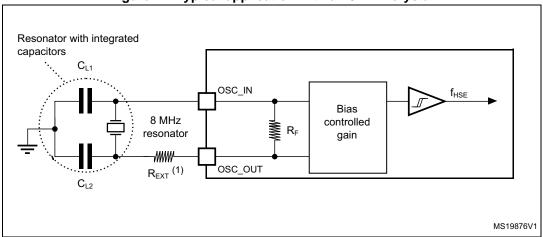
Figure 17. Typical application with an 8 MHz crystal
