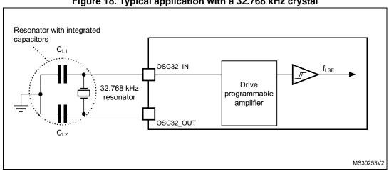
Figure 18. Typical application with a 32.768 kHz crystal
