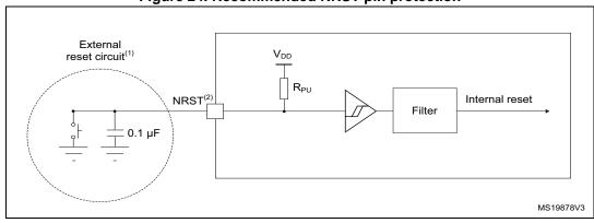
Figure 24. Recommended NRST pin protection
