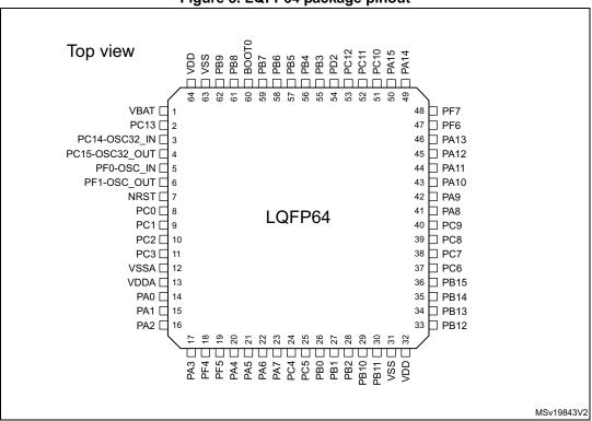
Figure 3. LQFP64 package pinout
