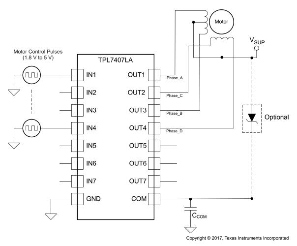
Figure 7. Stepper Motor Driver Schematic
