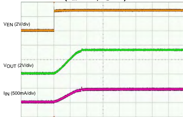
AP2280-1 Turn-On ( V_{IN}=3.3V, R_L=7\Omega )
