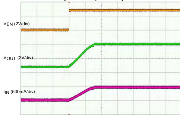
AP2280-2 Turn-On ( V_{IN}=3.3V , R_L=7\Omega )
