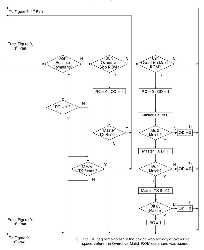
**NOTE**: For operation at overdrive speed, the DS28EC20 requires V<sub>PUP</sub> to be 5V ±5%.
