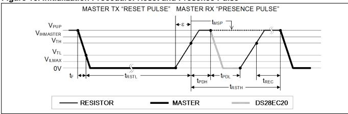
Figure 10. Initialization Procedure: Reset and Presence Pulse
