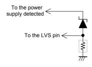
If the LVS pin is left open, the internal pull-down resistor will result in the IC seeing a ground level input, and the output will be turned off. Therefore, a voltage in excess of the LVS circuit clear voltage (about 4.35 V) must be applied to the LVS pin if the application does not use the undervoltage protection circuit. The maximum rating for the LVS pin applied voltage is 18 V.
