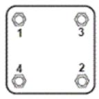
4. Apply no-flux solder to each pin of the TGA2814-CP. The component leads should be manually soldered, and the package cannot be subjected to conventional reflow processes. The use of no-clean solder to avoid washing after soldering is recommended.
