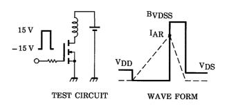
$$\begin{aligned} &RG = 25~\Omega \\ &V_{DD} = 90~V,~L = 7.01~mH \end{aligned} \qquad E_{AS} = \frac{1}{2} \cdot L \cdot I^2 \cdot \left(\frac{B_{VDSS}}{B_{VDSS} - V_{DD}}\right) \end{aligned}$$
