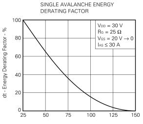
Starting T<sub>ch</sub> - Starting Channel Temperature - °C
