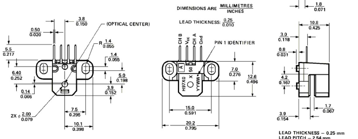
**Mounting Option #50 - Standard (Baseplane Mounting)** Contact Factory for Detailed Package Dimensions
