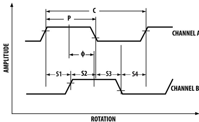
Pulse Width (P): The number of electrical degrees that an output is high during one cycle. This value is nominally 180°e or 1/2 cycle.
