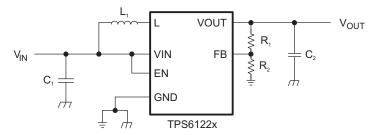
Figure 28. Application Circuit For Adjustable Output Voltage Option
