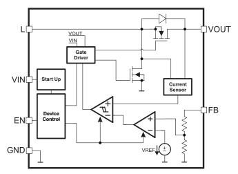
Figure 24. Functional Block Diagram (Fixed Output Voltage Version)
