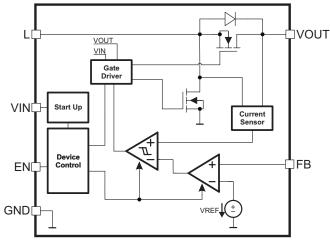
Figure 23. Functional Block Diagram (Adjustable Version)
