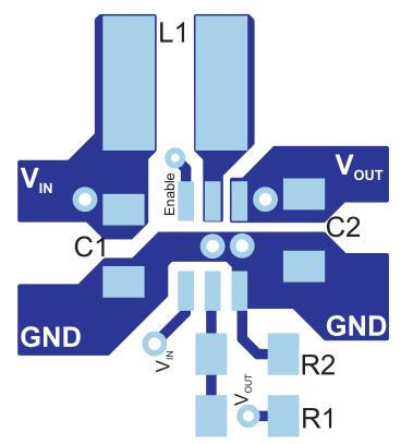
Figure 30. PCB Layout Suggestion For Adjustable Output Voltage Options
