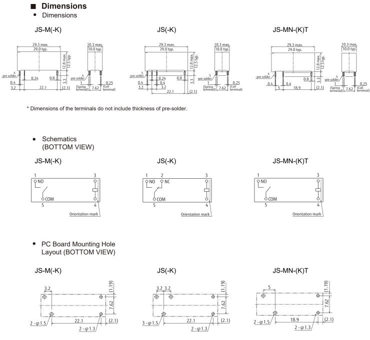
\* Tolerance of PC board mounting hole layout: ±0.1 unless otherwise specified.
