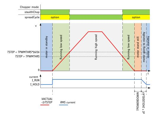
Figure 6.7 TPWMTHRS for optional switching to SpreadCycle
