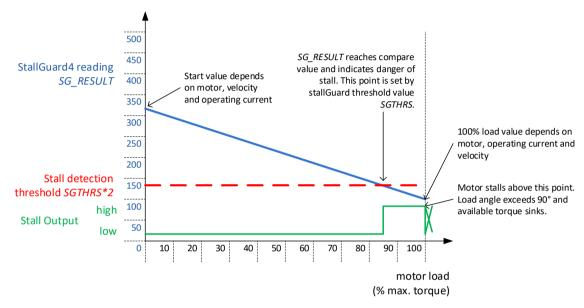
Figure 11.1 Function principle of StallGuard4
