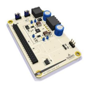
The TMC2209-EVAL is part of TRINAMICs universal evaluation board system which provides a convenient handling of the hardware as well as a userfriendly software tool for evaluation. The TMC2209 evaluation board system consists of three parts: STARTRAMPE (base board), ESELSBRÜCKE (connector board with several test points and stand-alone settings), and TMC2209-EVAL.
