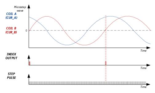
Figure 13.3 Index signal at positive zero transition of the coil B sine curve
