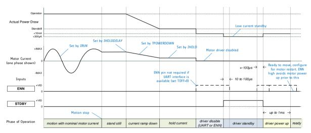
Figure 3.4 Switching to Standby and back On
