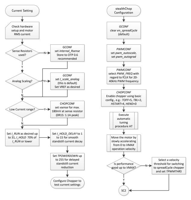
Figure 16.1 Current Setting and first steps with StealthChop
