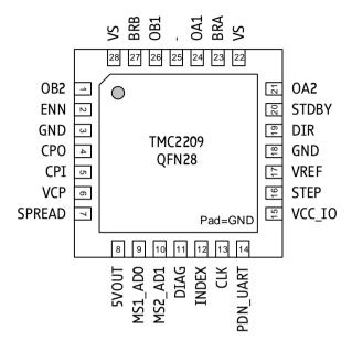
Figure 2.1 TMC2209 Pinning Top View - type: QFN28, 5x5mm², 0.5mm pitch
