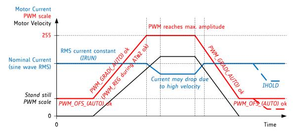
Figure 6.5 Successfully determined PWM\_GRAD(\_AUTO) and PWM\_OFS(\_AUTO)
