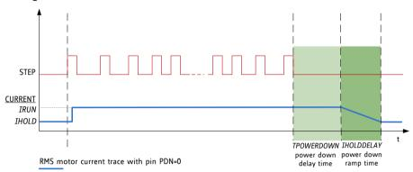
Figure 1.4 Automatic Motor Current Power Down
