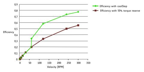
Figure 1.3 Energy efficiency with CoolStep (example)
