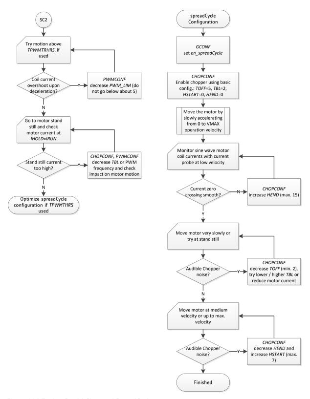
Figure 16.2 Tuning StealthChop and SpreadCycle
