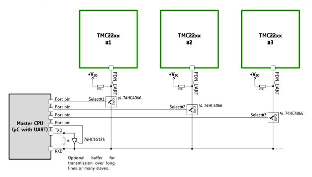
Figure 4.2 Addressing multiple TMC2209 via single wire interface using analog switches
