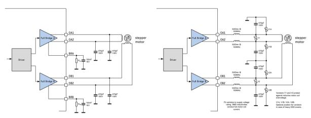
Figure 3.5 Simple ESD enhancement and more elaborate motor output protection
