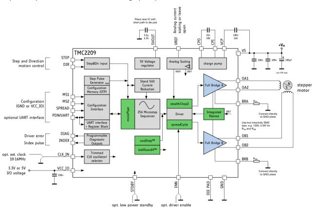
Figure 1.1 TMC2209 basic application block diagram
