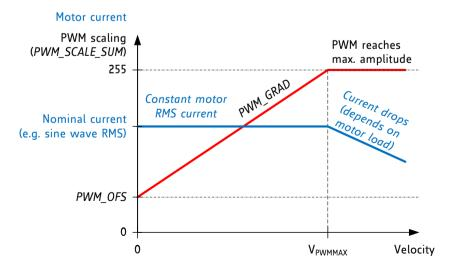
Figure 6.6 Velocity based PWM scaling (pwm\_autoscale=0)
