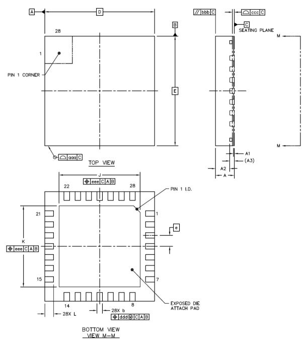
Figure 22.1 Dimensional drawings QFN28
