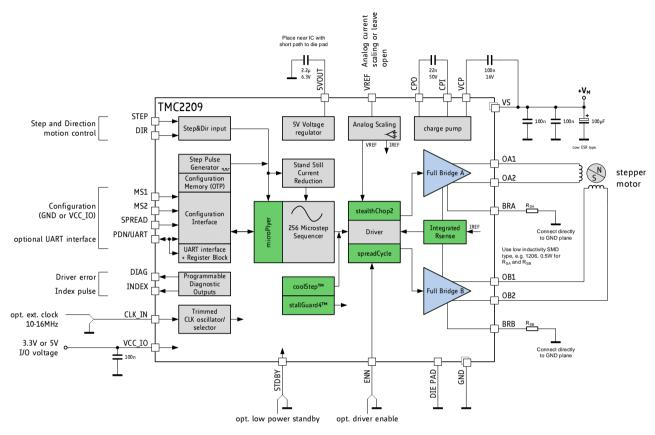
Figure 3.1 Standard application circuit
