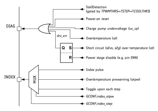
Figure 15.1 DIAG and INDEX outputs
