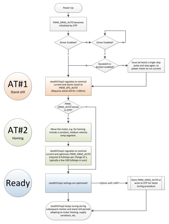
Figure 6.2 StealthChop2 automatic tuning procedure
