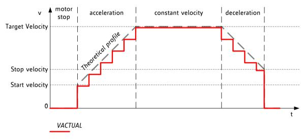
Figure 14.1 Software generated motion profile
