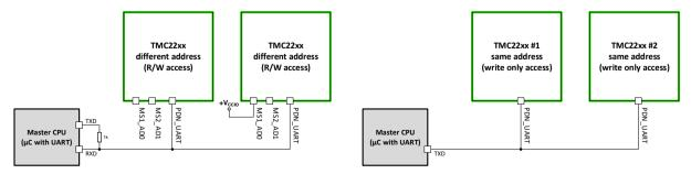
Figure 4.1 Attaching the TMC2209 to a microcontroller UART
